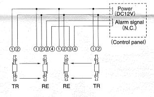
4) When two sensors are stacked and connected to the same line.
