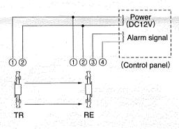
3) When two or more sensors are connected to separate lines.
