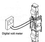
TReverse the procedure, i.e. attach shading plates to upper optics of transmitter and receiver and repeat adjustment.
