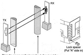
Place the covers on the beam line before insert the lock spacer so as to get the same beam strength as the covers are attached
